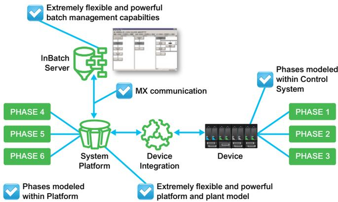
This platform integration simplifies building a common real time data model across all manufacturing operations which may span across receiving, batching, filling, packaging and shipping. InBatch execution information is available to be directly leveraged by other software functionality such as Wonderware Historian or by Wonderware MES Software.
