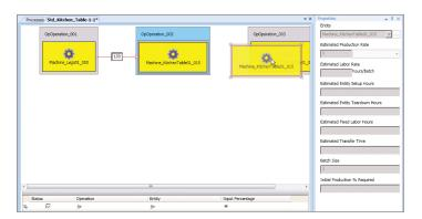
The process model allows defining and linking the operations, equipment, BOM and setup specifications, routings and flow of materials between operations and the data capture requirements for each operation or step within a process.
