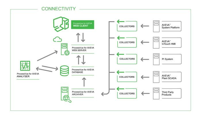
There is no complex engineering required to integrate ProcessVue for AVEVA, a wizard with 'out-of-the-box' configurations simplifies the process, reports can be generated within minutes. A suite of connectivity drivers facilitate seamless connectivity to AVEVA and third party products, providing a centralised system for all alarm and event data and a unified view across previously siloed systems.
